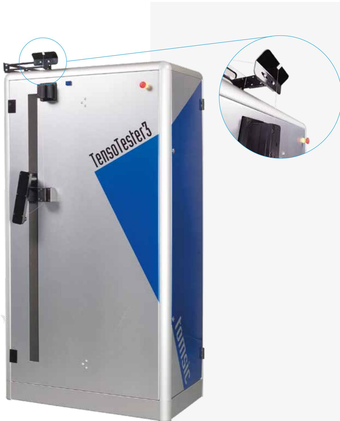
Single-Position Automatic tensile strength tester for yarns.
